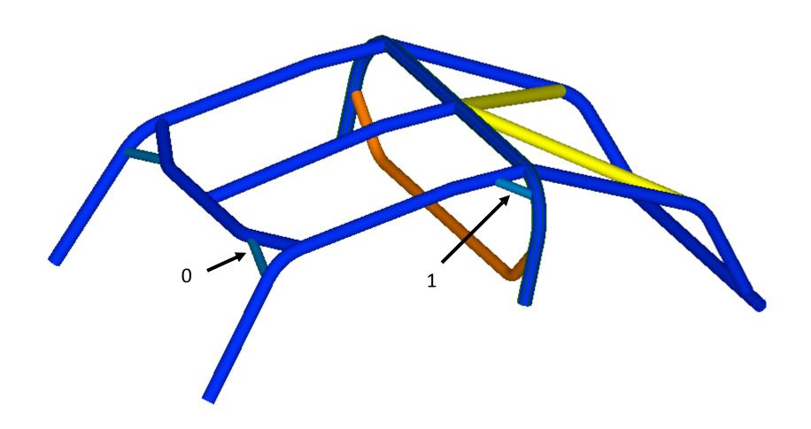
Part Numbers engraved within 3" of the end of part Passenger side parts are followed with a M (for Mirrored)
