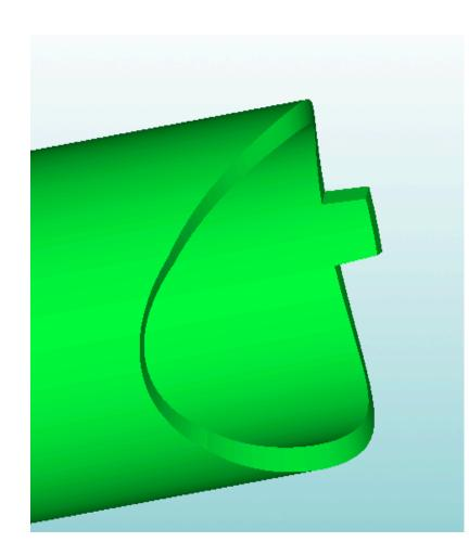
Slot and tab cuts will locate the parts with these features.
