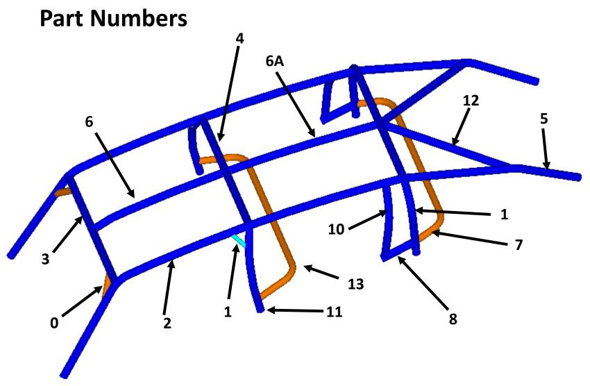
Part numbers are engraved within 3" of the start of the part. There is no Part 9 Passenger parts are followed with an M (for Mirror)
